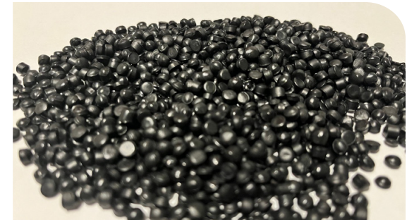
The final result is post-consumer resin pellets ready to be turned into new products.
