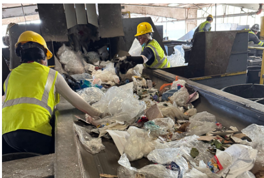
Sorting film and flexible packaging for recycling at the Valemi facility.
